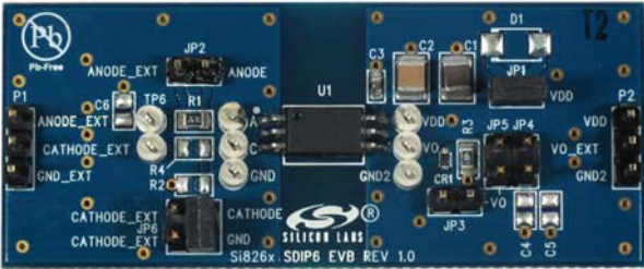
Figure 3. Si826x SDIP6 Evaluation Board Overview
