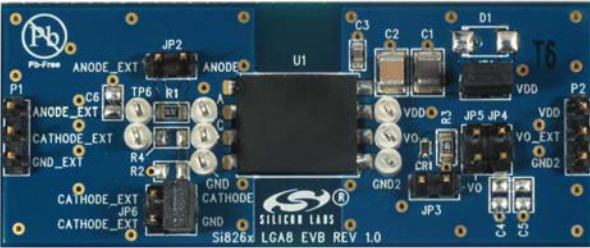
Figure 4. Si826x LGA8 Evaluation Board Overview
